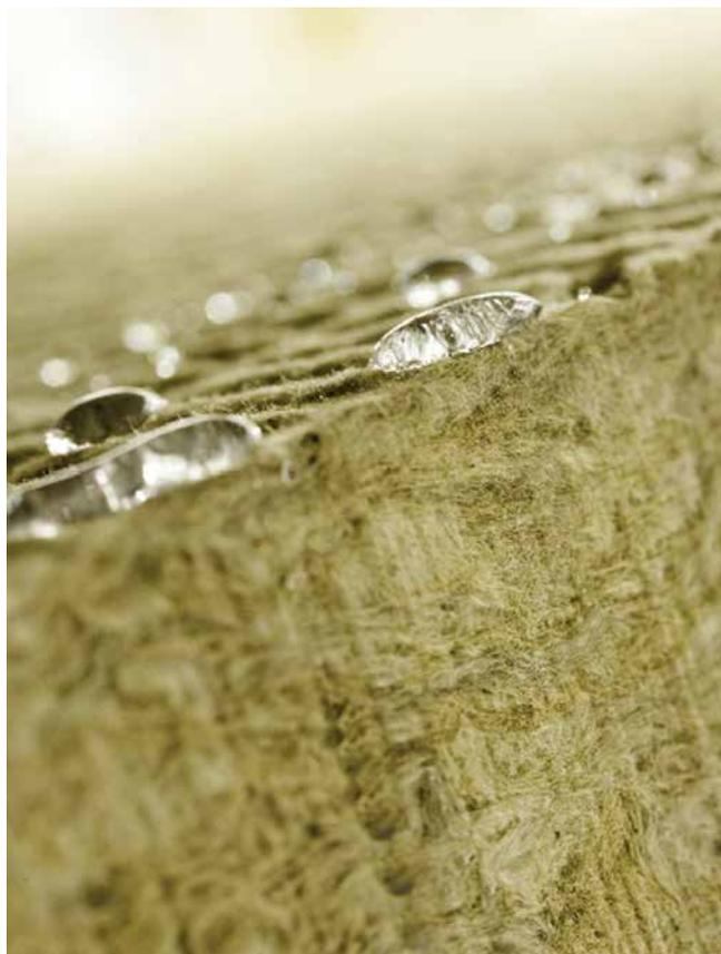
This unique vapor permeable quality of ROCKWOOL's curtain wall insulation allows for an increased potential for drying without trapping water in the wall assembly.
