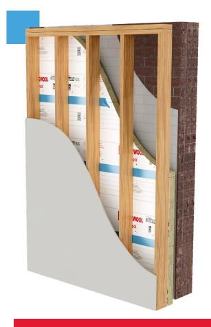
Smartrock has recieved ICC-ES validated product acceptance within ESR-5374 and AC 566 for installation on the interior side of exterior mass wall assemblies.\*
