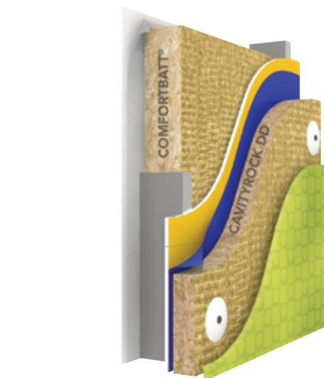
In the ROCKWOOL BEDR™ Wall system, COMFORTBATT® Steel Stud insulation allows builders to achieve a thermal value of R24 and offers superior acoustical performance in comparison to traditional steel stud wall cavities.
