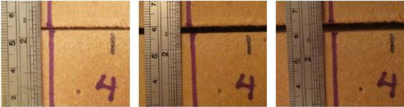
Figure 3: Photographs of measurement location for polyisocyanurate during Phase 2a, cycle #1, #3 and #6 at -18°F (-28°C)
