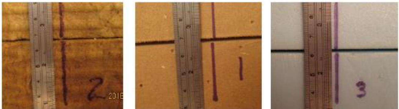
Figure 4: Photographs of all three insulation materials (from left: ROCKWOOL TOPROCK DD, polyisocyanurate and XPS) at end of Phase 2a testing (once equilibrium was achieved) showing permanent dimensional changes.
