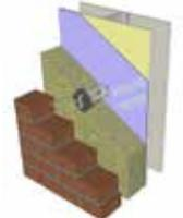
Masonry ties with semi-rigid insulation. The tie supports here provide only lateral resistance support, not gravity load (supported at the base of the veneer).
