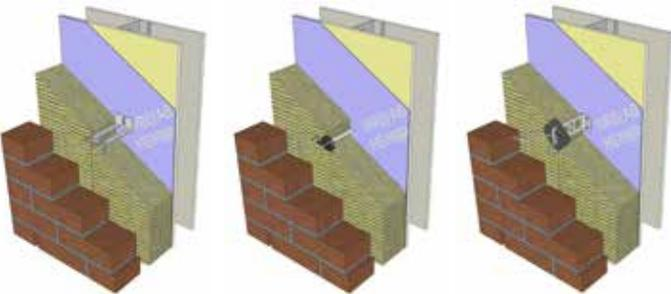
Examples of alternate masonry ties installed through ROCKWOOL CAVITYROCK® insulation.
