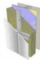
Long screws through rigid insulation utilizing continuous vertical strapping to create a truss cladding support system. Cladding attached to strapping on exterior of insulation.
