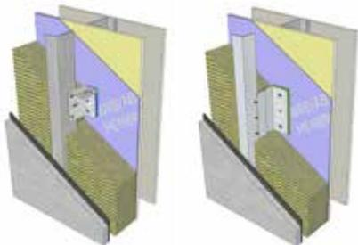
Additional examples of thermally isolated galvanized steel clips where low-conductivity pads are used to reduce the heat flow through each clip. Note that the best performance arises when the continuous girts attached to the clips are entirely outboard of the insulation and do not cut through it.
