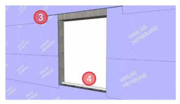
This installation is for an aluminum window frame (non-curtain wall) in punched configuration. Detail could be modified slightly based on window type.
