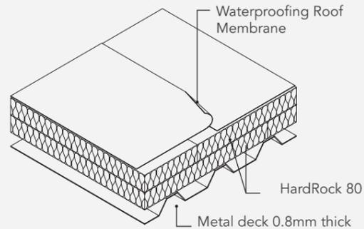
With the high density of ROCKWOOL HardRock roofing boards and the structure of the product, it provides the added mass necessary for effective sound insulation of membrane roof system. Additionally, the single-ply roof membrane coupled with ROCKWOOL stone wool insulation effectively minimizes rain impact noise on the roof system.
