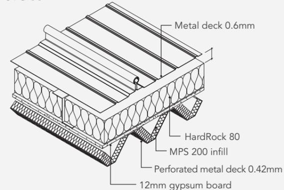
Laboratory testing have proven the added advantage of Hardrock roofing boards in metal roof system. With the high sound absorption characteristics of ROCKWOOL roofing boards, it provides an effective damping of sound resonance within the roofing system. To enhance the quality of sound, ROCKWOOL stone wool infills can be introduced inside the trapezoidal of the perforated metal deck to provide added sound absorption for reverberation control.
