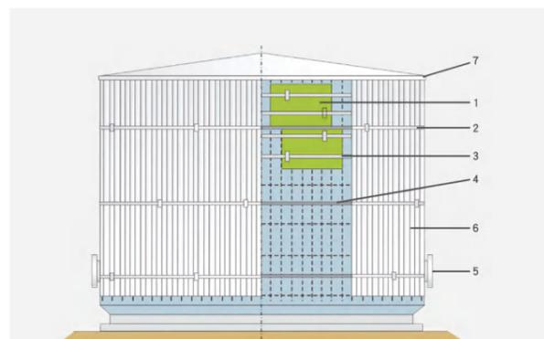
1,RockTech Slab 2,Self-adhesive foil tape 3,Self-adhesive foil tape
