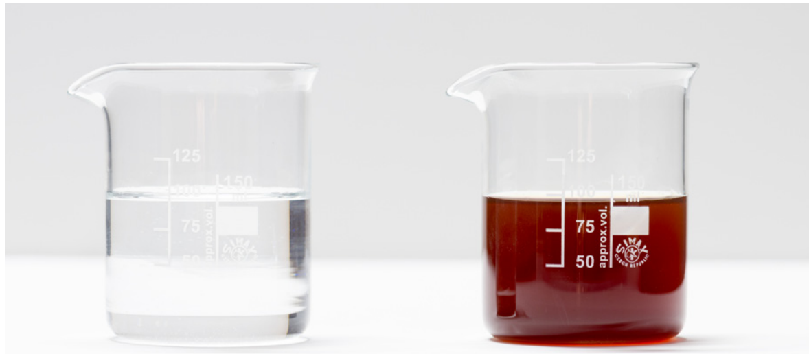
Figure 6. First flush drain water from GRODAN substrate (left) compared to coco (right).
