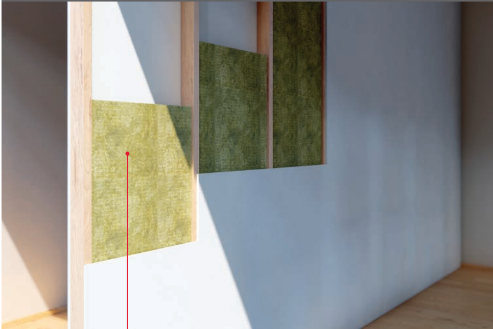
Sound Insulation Slab
