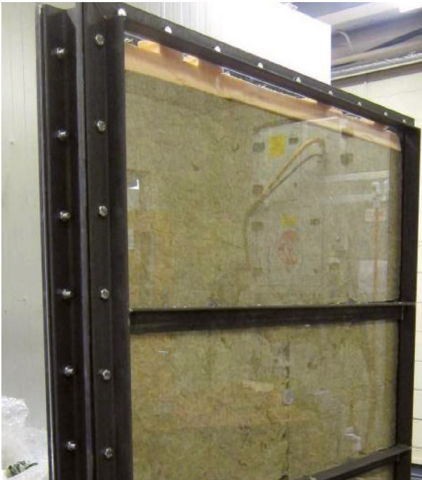
Figure 1: ROCKWOOL Cavity insulation in a flooding test rig developed by Glasgow Caledonian University.
