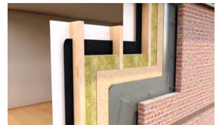
Timber Frame Wall
